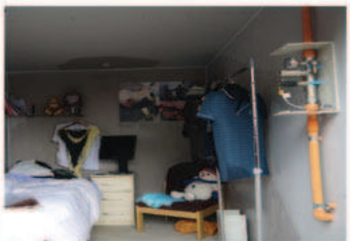
Fire extinguished with a mist system 2-minutes after it had started. (Slight water damage and only a small amount of fire damage).
